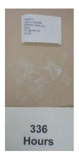
Following its ageing period of 336 accelerated ageing hours (calculated to around 7.3 months at 20°C), the translucent PE film sample containing Reverte<sup>™</sup>, referenced Pamuk Ambalaj Beyaz Renk Atlet Poset, can be seen to have lost all of its significant physical properties, is exhibiting extreme friability and breaking up when handled.
